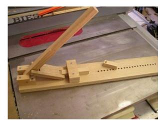
Here is the finished unit. The last thing that I did was to use CA glue to attach a piece of thin (1/16") plexiglass to both the end of the slide and the end of the stop. This way, the sharp point of the pen tips will not damage the
