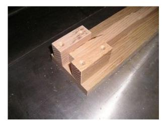
The first step was to cut the base. I cut it ~4 inches wide and 24 inches long. Then I made a handle that was 3/4 inch square and 14 inches long. I used the router to round over the edges on the first 7 inches. I placed the two bottom lever blocks on each side of the handle and screwed them to the base.
