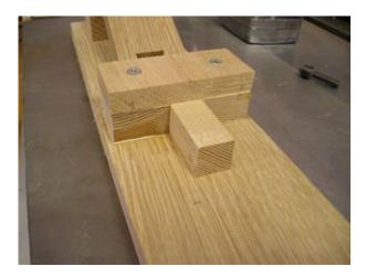
To ensure that the slide runs parallel to the base, I've added a slide guide. It's just two blocks (one on either side of the slide) and a top. The screws go all the way into the base. I made the length of the slide guide so that the joiner board barely hits it when the handle is completely down and the slide sits slightly proud of the guide when the handle is up.
