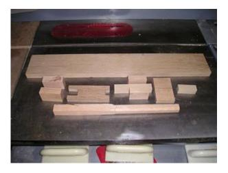
Here are all the parts that I cut to make the unit. They are mostly 3/4" stock with the exception of the joiner board (connects the handle to the slide) and the top to the slide guide.
