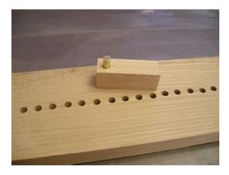
To work, the slide must press against something, so I've created a stop using a peg and a set of holes set 1/2" apart. I've seen stepped stops but I like the ablitity to move the press board in small increments.
