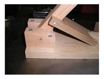
Now I've attached the joiner board to the handle with another steel pin. You can also see that I've decided to notch the bottom lever blocks to give me more clearance. The key to the entire jig is that the distance from the bottom to top pins on the handle is equivalent (or close enough) to the throw of the slide.
