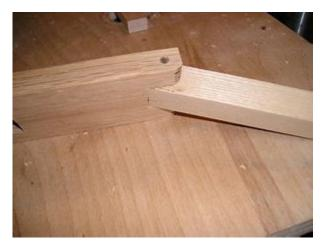
Next I took my 3/4 inch square slide and attached it to the slide joiner board by drilling it and inserting a length of the steel pin. I used a hacksaw to cut the steel pin. You can also see that I've rounded over the end of the joiner board with a belt sander.
