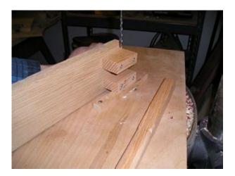
Once the bottom lever blocks were installed. I used the drill press to drill a hole through the blocks and the handle. I planned to use 3/16 inch steel rod as my lever pin. I bought 3 feet of it from the local hardware store.
