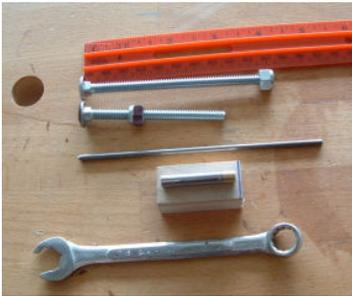
Pictured above are simple jigs to assemble or disassemble 7mm slimline pens.
