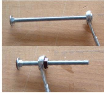
Jig for pen assembly. Spin on a nylon stop nut about a 1/2" to cut the threads. (top photo) then remove it and spin it on backwards to the depth you will set the transmission. (bottom photo) (approx 1-11/16") from the base of the nut to the tip of the bolt. Once set you will be able to install the transmission to the correct depth every time.
