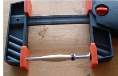
For use: simply insert the carriage bolt with stop nut in the tip end of the pen, and the transmission in the other end and press until the transmission bottoms out on the bolt. If you are doing production work this will really speed up the process. (Note this is the reverse assembly you may be used to.) Assemble the clip & cap as usual into the upper barrel of the pen and set aside. See next photo for tip assembly.
