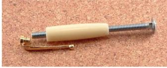
To remove the clip from the barrel, insert a 4" carriage bolt into the barrel until it bottoms on the clip cap. Hold the barrel tightly in your hand and tap the bolt with a hammer. This is the same procedure as for the tip.
