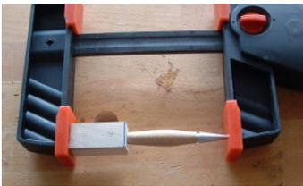
Cut a hardwood block 3/4 x 3/4 x 1 - 7/8" and drill a 7mm hole in it. Slide the block over the transmission and set the pen tip. Install the pen refill and slide the upper barrel on and you are done. This hardwood block will also be used for disassembly. These jigs will only set you back about \$3 bucks, and about 10 min. of your time.
